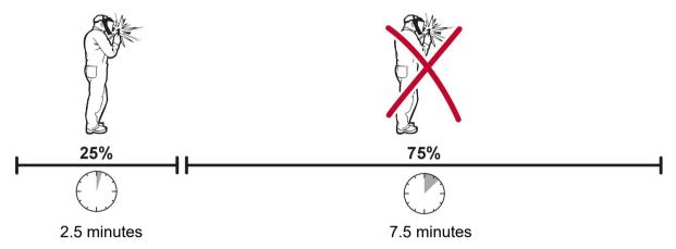
A different combination of duty cycle and welding current can be selected. Use the graphs below to determine the correct duty cycle for a given welding current.
